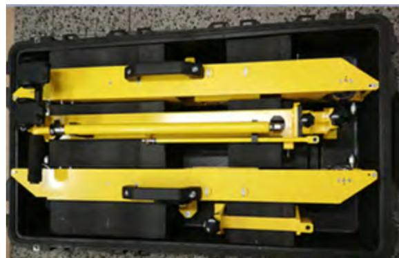
*For easier transportation the trolley can be easily fold*
