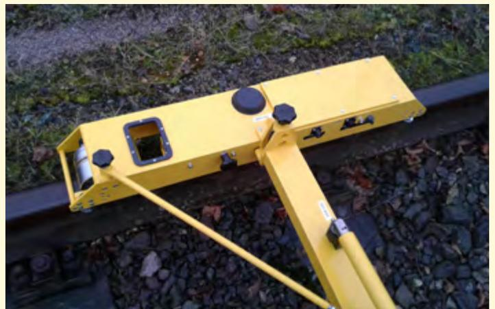
The **DOUBLE GEKON - K Trolley** is able to measure a series of continuous track sections, evaluate the acquired data and compute the results being complied with the standard EN 13231-3. For the measurement, the **DOUBLE GEKON - K** uses two versines with laser sensors placed vertically to the longitudinal axis of the rail. The measurement can be taken any speed of range 0 - 7,2 km/h.
