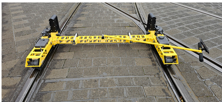
Two measurement units and rail profile cameras (one on each side of the trolley).
