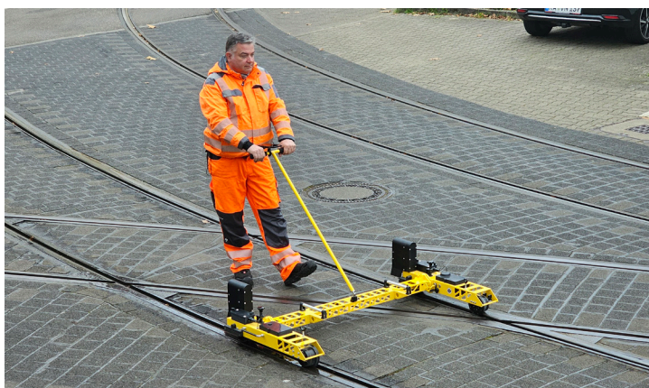
Suitable for tram track switch measurement
