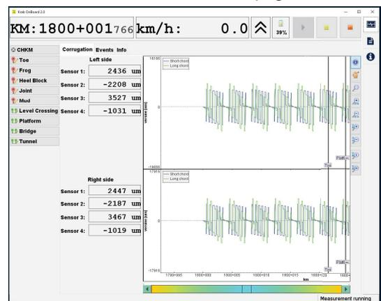
Krab OnBoard 2.0 running - measured signals
