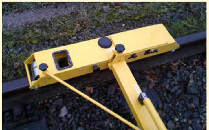
The **DOUBLE GEKON Trolley** is able to measure a series of continuous track sections, evaluate the acquired data and compute the results being complied with the standard EN 13231-3. For the measurement, the **DOUBLE GEKON** uses two versines with laser sensors placed vertically to the longitudinal axis of the rail. The measurement can be taken any speed of range 0 - 7,2 km/h.
