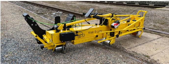
For easier transportation the trolley can be easily folded
