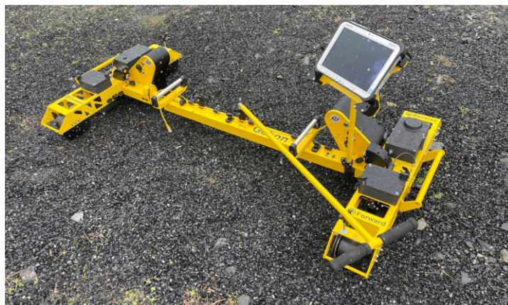
Double rail measurement version with two rail profile scanners
