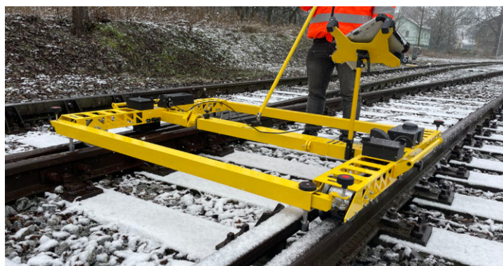
Equipped with "stay on track" elements for passing switches
